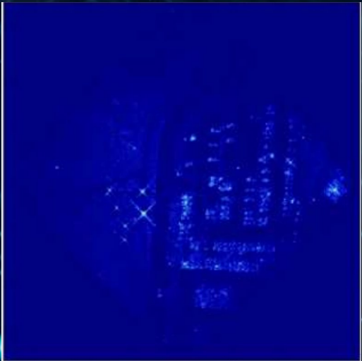
Video radar reconstruction of the parking lot scanned by an airplane
